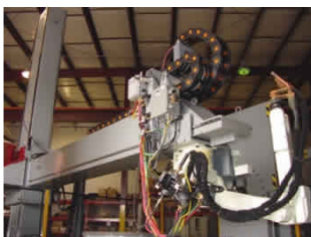
Robot—9 Axis Arc Welding
