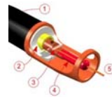
Figure 10-46. Typical semiautomatic gas-cooled, curved-neck gas metal arc welding gun.
