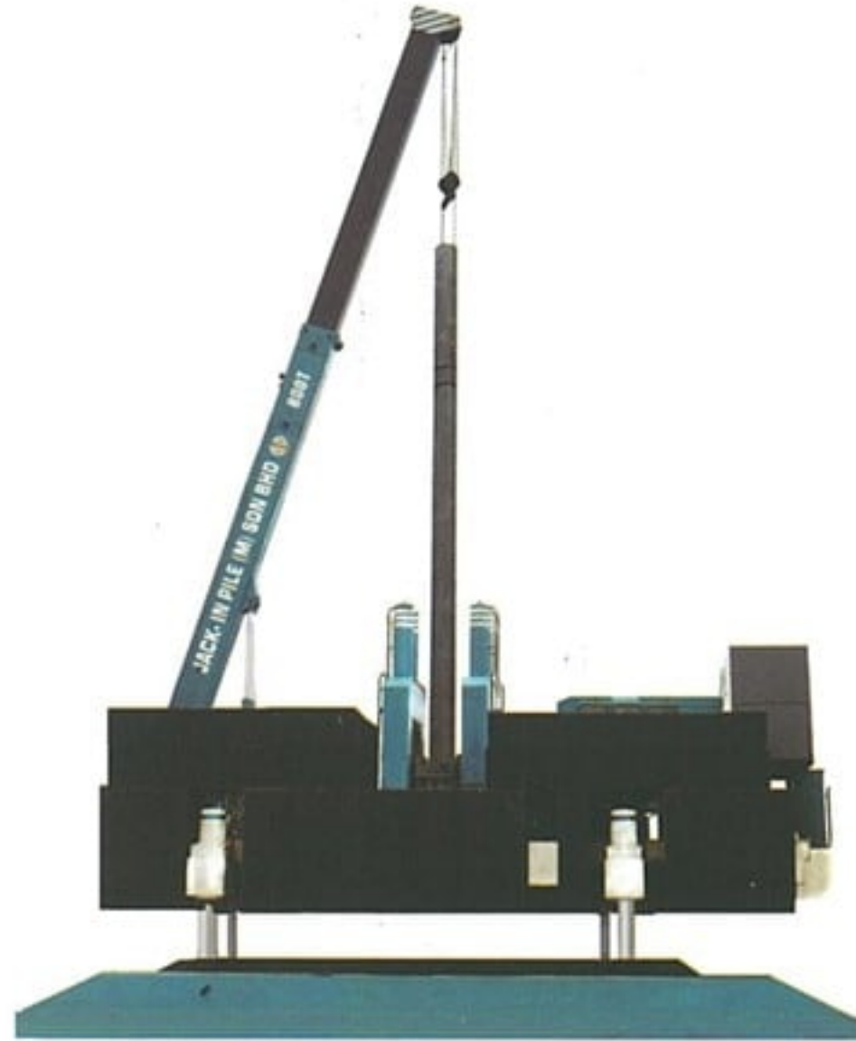
800 Tons Hydraulic Jack-in machines with crane
