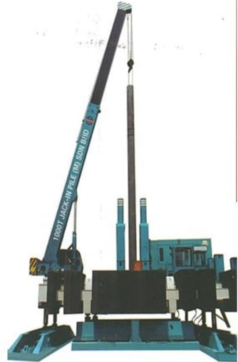
1000 Tons Hydraulic Jack-in machines with crane
