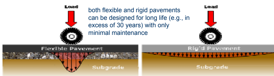
Figure 1: Rigid and Flexible Pavement Load Distribution 20/09/54 01203571 pavement design
